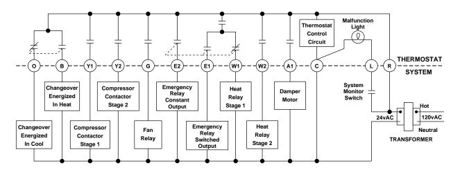
Figure 4. Typical wiring diagram for single transformer systems
